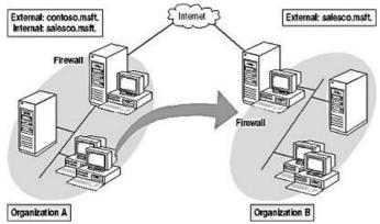
**Figure 9.7** *Example where an organization's internal domain namespace is identical to another organization's external domain namespace*
