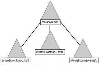
Figure 9.24 Diagram of the university's existing domain namespace
