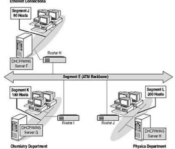
**Figure 9.27** Existing network at the Chemistry and Physics buildings (assume that these buildings have the same network configuration)
