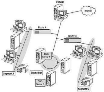
Figure 9.17 Example of how multiple DNS servers with replicated zones provide enhanced availability
