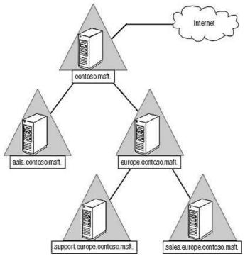
Figure 9.10 Scenario that illustrates the appropriate selection of DNS zones in the design
