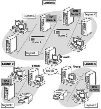
Figure 9.16 A scenario that illustrates the proper methods for preventing unauthorized user access to DNS servers
