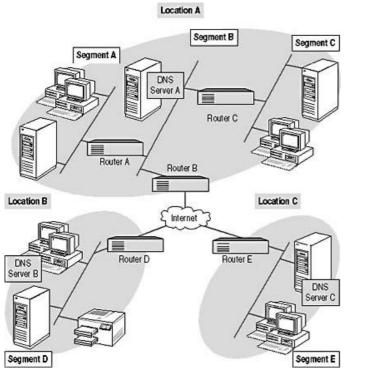
Figure 9.11 Scenario that illustrates the appropriate placement of DNS servers
