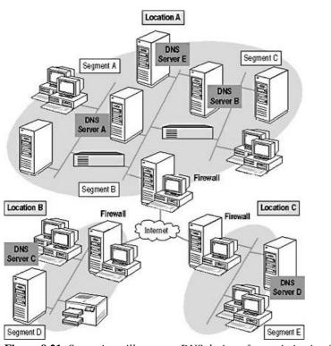
Figure 9.21 Scenario to illustrate a DNS design after optimization for performance
