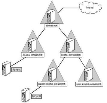
Figure 9.5 Example where an organization has a combination of external and internal domain namespaces
