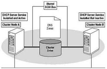
Figure 9.18 Components in a Windows Clustering server cluster
