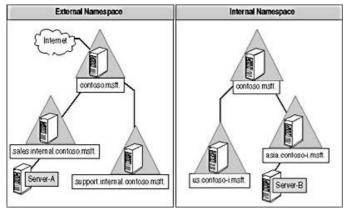
Figure 9.6 Example where an organization has separate external and internal domain namespaces
