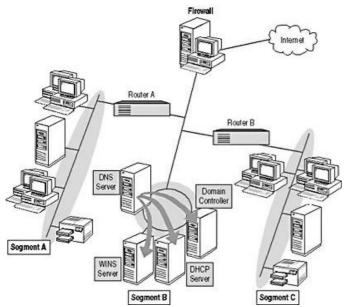
Figure 9.1 The interaction between DNS and other Windows 2000 networking services
