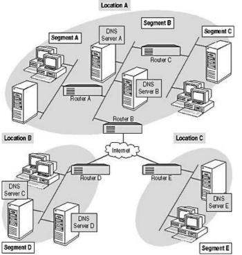
**Figure 9.3** Scenario that incorporates DNS services in Windows 2000 with BIND DNS servers <u>3.4</u>
